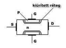
The potential of the G (GATE) contact can be used to change the thickness of the depletion region, i.e. the conductivity of the conduction channel between the S (SOURCE) and D (DRAIN) contacts can be controlled.  $\rightarrow$  TRANSISTOR – EFFECT
