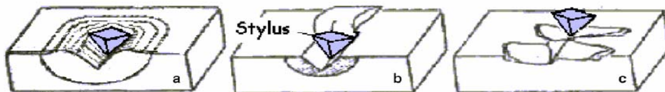
Fig. 1. Material loss mechanisms: (a) micro-ploughing, and (b) micro-cutting (c) micro-cracking.
