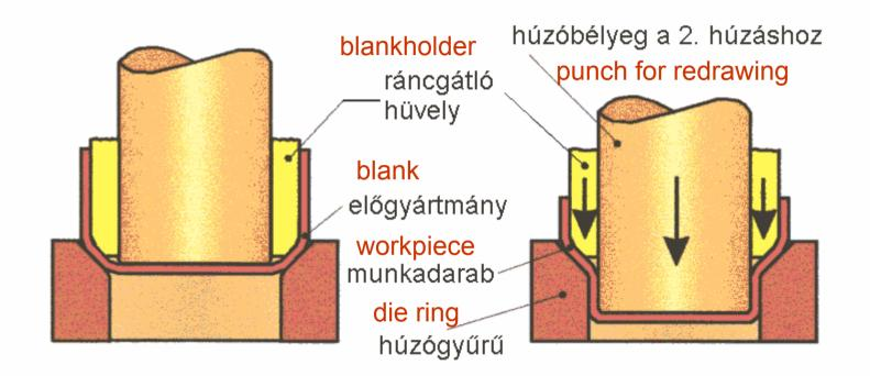
Final shape of a container can be reached by more drawing steps, these operations are called as redrawings
