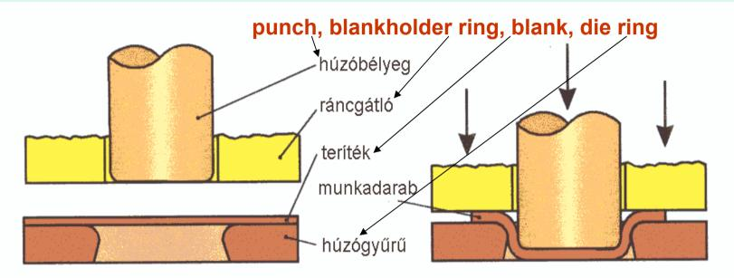
Deep drawing of metal sheet is used to form containers
