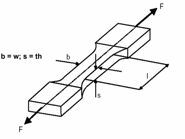
F ... Tensile force b ... Specimen width s ...Specimen thickness I ... Reference length
