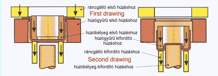
More drawing operations can be combined into one tool using multiple ram system in a hydraulic press
