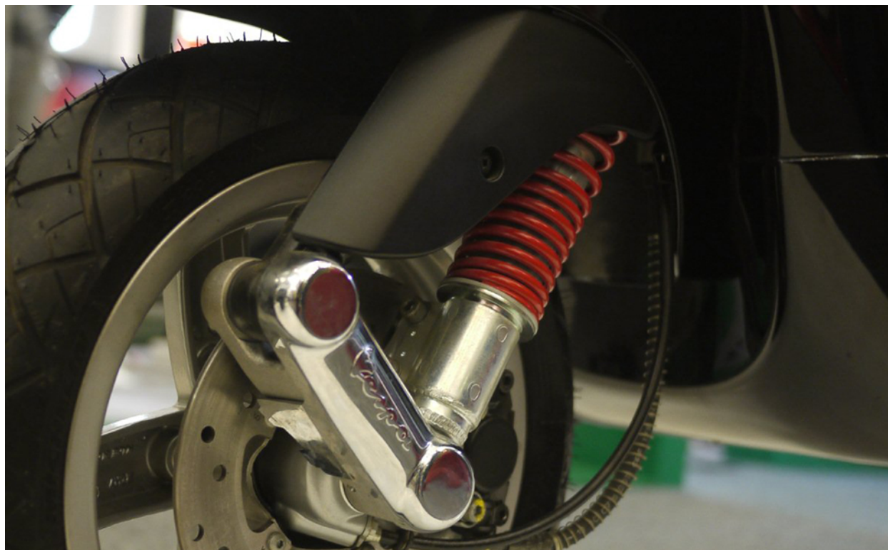
Figure 7.1 A motorcycle suspension system is an example of a damped spring-mass system. The spring absorbs bumps and keeps the tire in contact with the road. The shock absorber damps the motion so the motorcycle does not continue to bounce after going over each bump. (credit: nSeika, Flickr)
