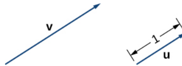
Figure 2.17 The vector \mathbf{v} and associated unit vector \mathbf{u} = \frac{1}{\| \mathbf{v} \|} \mathbf{v} . In this case, \| \mathbf{v} \| > 1 .
