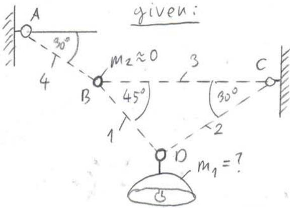
task: If the tension in each of the four wires is not allowed to exceed 600 N, determine the maximum mass of the chandelier that can be supported.
