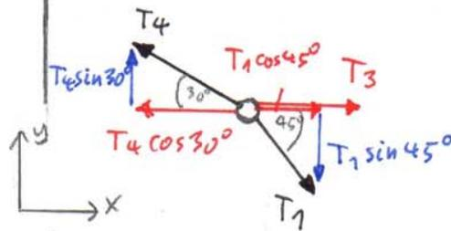
2 EE  $\Sigma F_x = 0 \Rightarrow 1) T_2 \cos 30^\circ - T_1 \cos 45^\circ = 0$
