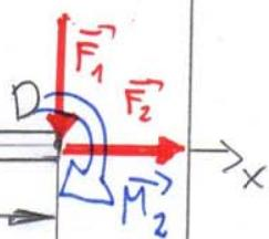
$$\begin{aligned} \text{a)} \quad \sum F_x &= F_2 + F_3 \sin L = 403.2 \text{ N} \\ \sum F_y &= -F_1 + F_3 \cos L = -21.4 \text{ N} \end{aligned} \quad \left\{ \begin{aligned} \sum \vec{F} &= \sum F_x \vec{i} + \sum F_y \vec{j} = \\ &= (403.2 \vec{i} - 21.4 \vec{j}) \text{ N} \end{aligned} \right.$$
