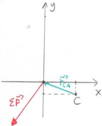
$\Sigma \vec{M}_C = \vec{r}_{CA} \times \Sigma \vec{F} + \Sigma \vec{M}_A = *$
