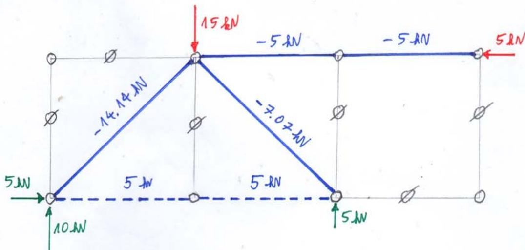
Calculation of  $N_7$  with method of sections:
