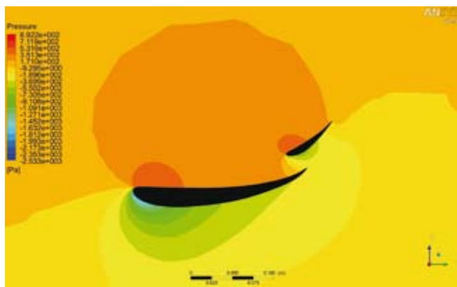
Figure 23: Pressure and velocity contours over the rear wing, deflecting of upper wing
