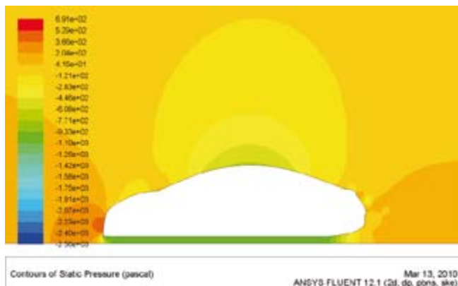
Figure 7: Static pressure contours over the initial car geometry (case one)
