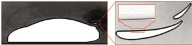
Figure 4: Finite volume mesh of the second case of car geometry (redesigned geometry)
