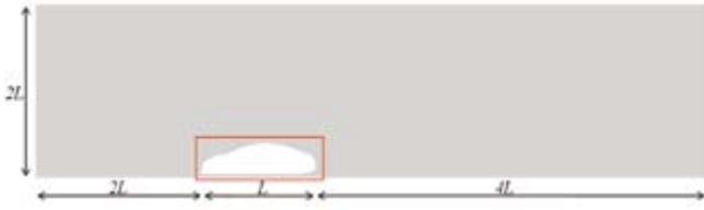
Figure 2: Dimensions and discretization of 2D domain
