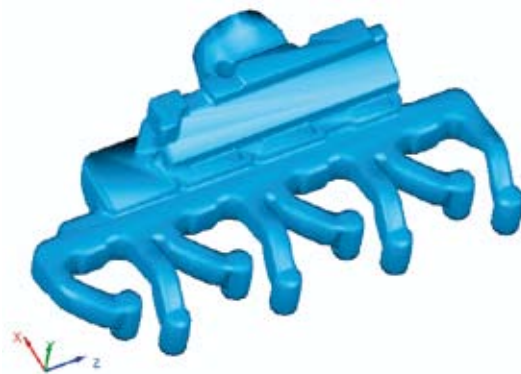
Figure 1. 3D CAD model of the intake manifold and ports
