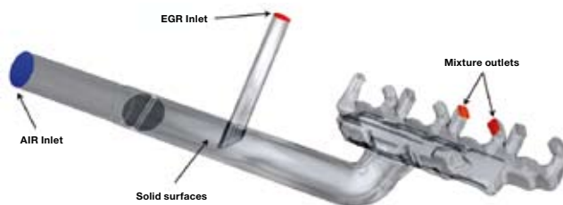
Figure 5. Simulation model with boundaries
