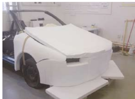
9. Model fabrication and preparation of laminating molds (scale 1:1)
