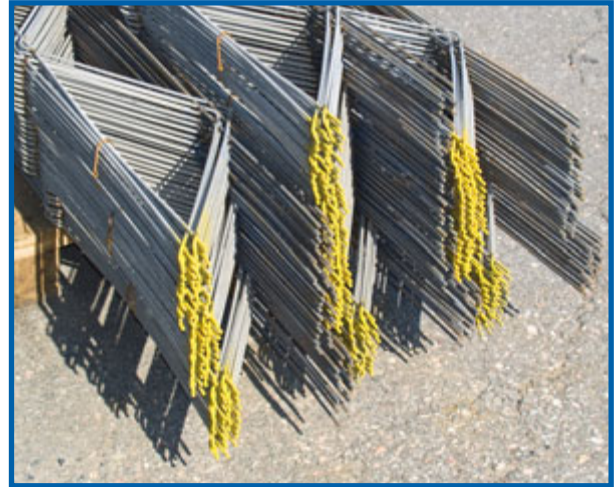
Figure 2. Stainless rebar of PD tie is marked with yellow.
