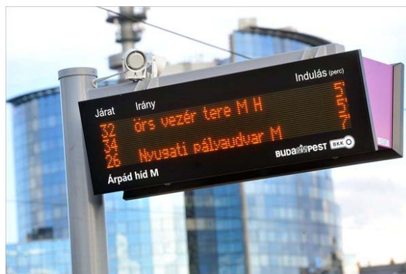
Fig. 34: Real-time information display to be installed at Kőbánya-Kispest as well (Source: BKK)
