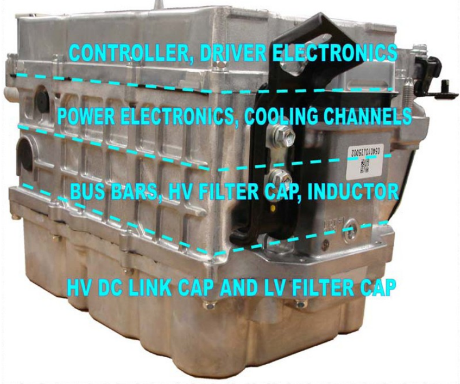
Fig. 2.3. Compartments of the LS 600h inverter and converter assembly.
