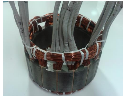
Fig. 3. The photo demonstrates the 1 st version of divided coiled stator.
