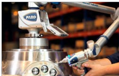
7-axis arm with rotating "wrist"
