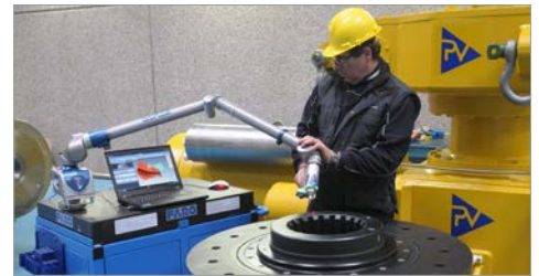
Reverse engineering using an arm and laser scanner
