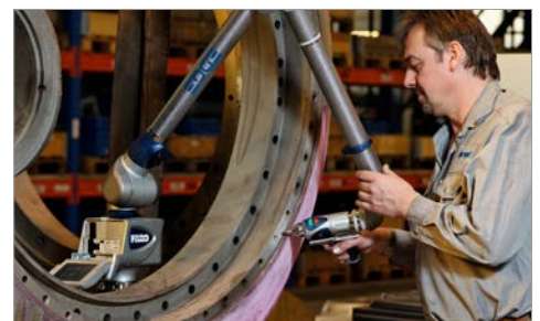
Dimensional analysis using an articulating arm
