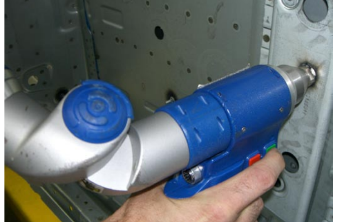
The measurement technician moves a sleeve over the bolt, which means that he does not have to touch it.
