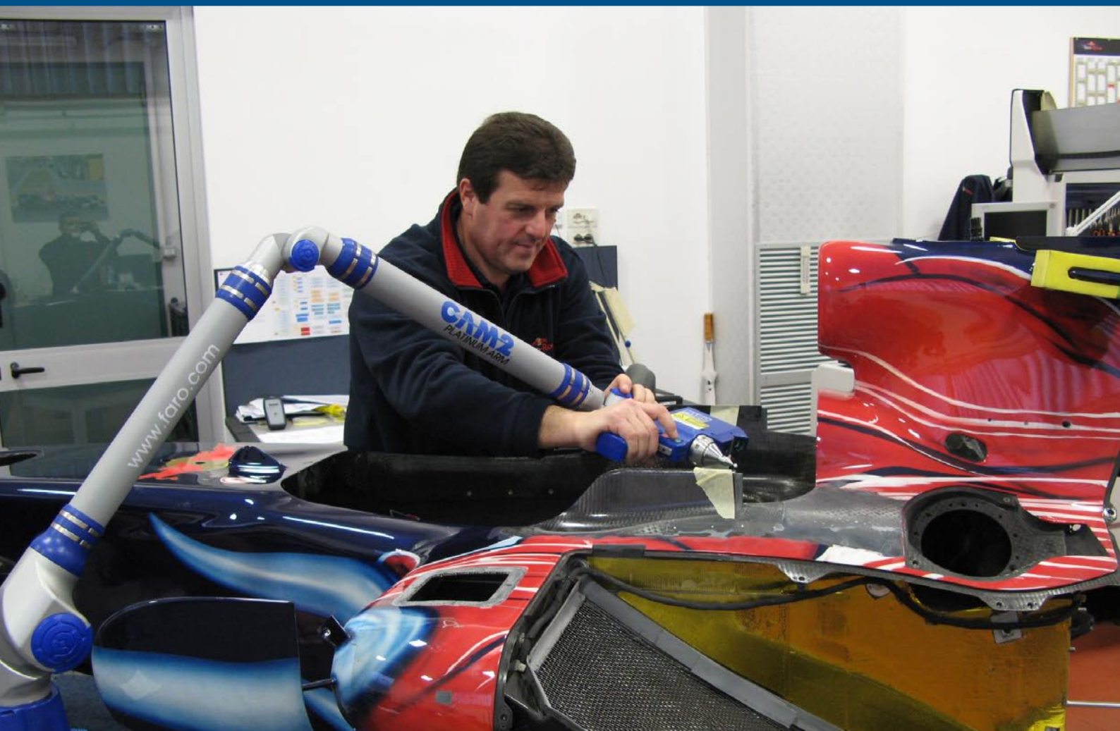
The FARO Laser ScanArm is being used to measure the wing profiles, the bodywork and the gearbox housing
