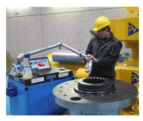
Reverse engineering can shortcut product development time. It quickly captures a product in 3D digital form and exports the data for rapid prototyping, tooling, or manufacturing.
