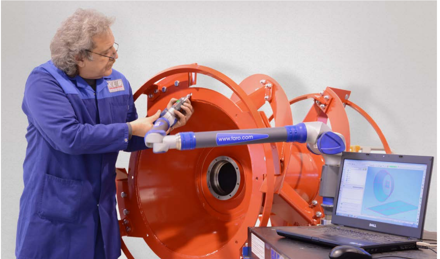
Quality assurance at KLB Blech in Form GmbH with the help of the FARO Fusion
