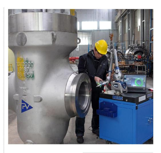
>> several consultations with FARO, the company chose the FARO Edge ScanArm (i.e. a FARO Edge measurement arm with a Laser Line Probe), equipped with CAM2 Q and Geomagic Qualify software.
