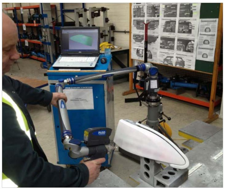
Laser scanning rear lamp cluster for comparison to CAD model.
