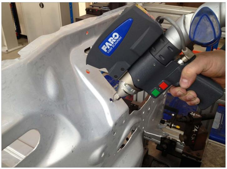
Inspecting thickness of body panel using the ceramics stylus.
