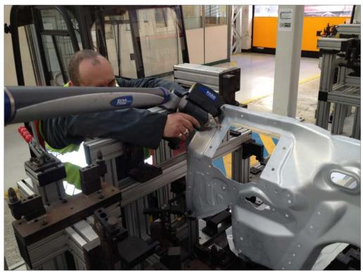
Confirming hole diameter & position to CAD.
