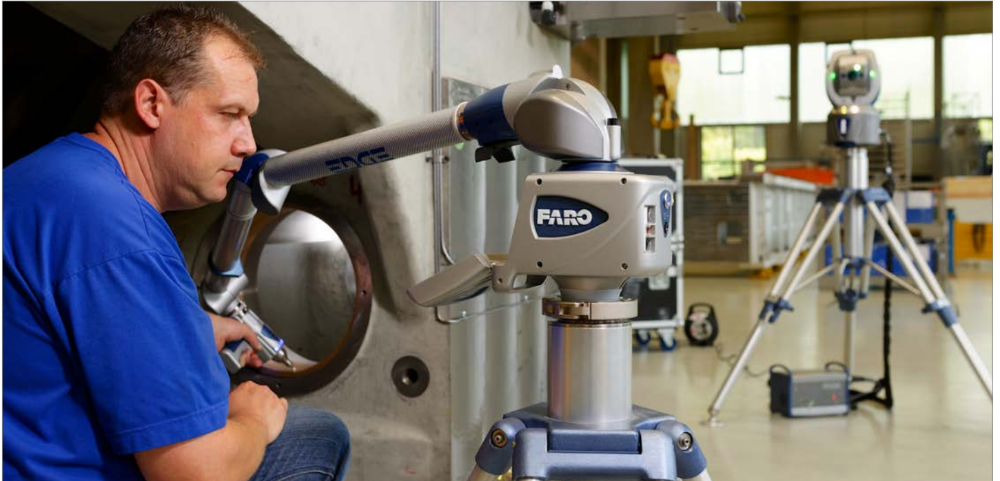
The combination of FaroArm and Laser Tracker enables extremely flexible measurement.
