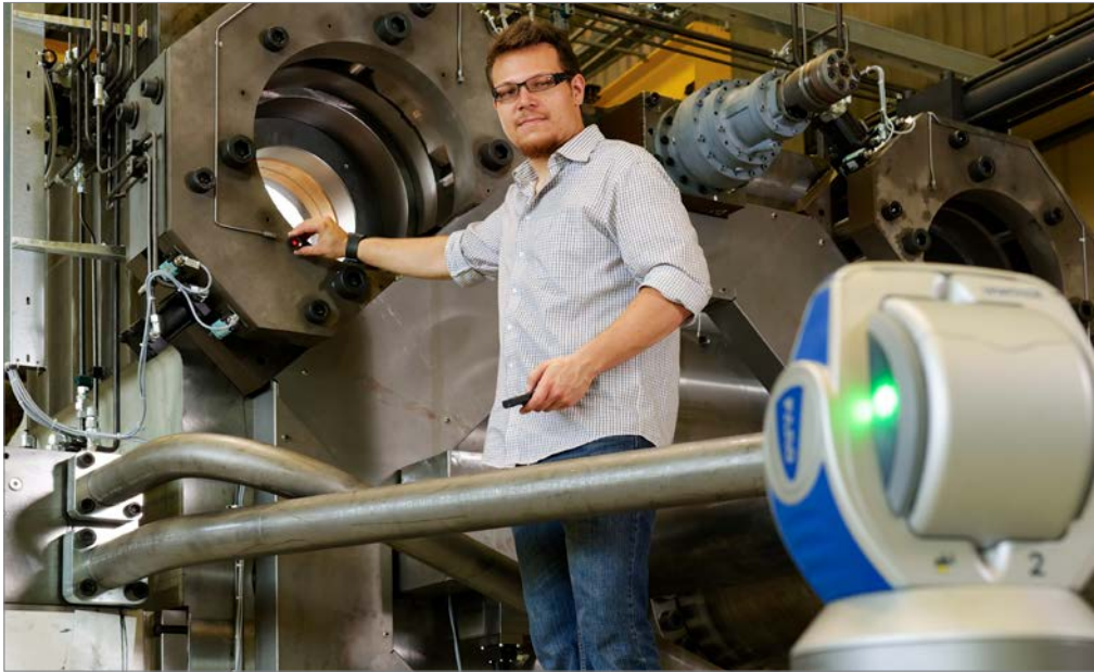
The Laser Tracker has become virtually indispensable in the assembly of large machines.
