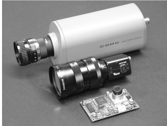
FIGURE 19.111 Three solid state cameras are shown. The nearest is an inexpensive single board camera with a CMOS sensor and 4-mm lens. The middle one is a miniature CCIR interline frame-transfer CCD camera, dwarfed by the 9.5- to 75-mm C-mount zoom lens. The rear camera is a high quality Cohu 4712 monochrome frame-transfer CCD camera fitted with a 16-mm C-mount lens and 20-mm extension tube.
