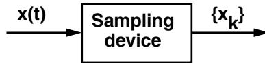
FIGURE 23.16 A continuous-time signal x(t) and a sampling device that produces a sample sequence \{x_k\} .
