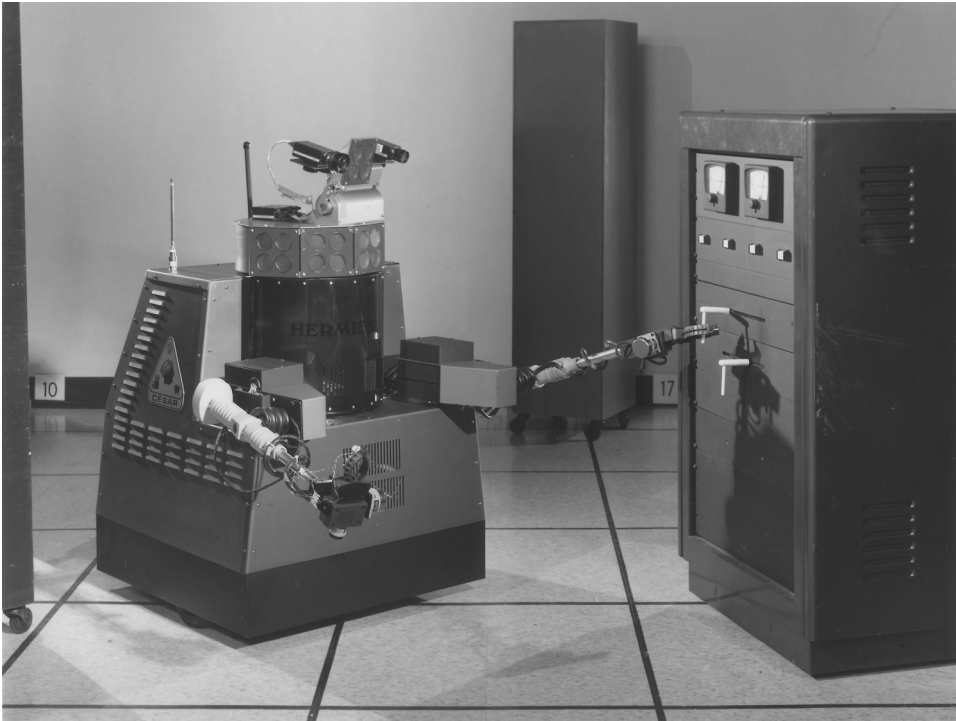
FIGURE 19.83 HERMIES IIB employed an active stereoscopic ranging system with an external laser source that could be used to designate objects of interest in the video image (courtesy Oak Ridge National Laboratory).
