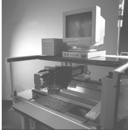
FIGURE 22.1 An optical inspection system for printed circuit boards. (Used by permission " CyberOptics Corporation 2001, all rights reserved.)
