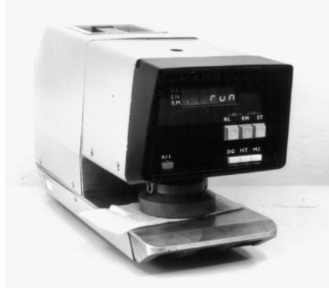
FIGURE 4.3 Example of a small mechatronic system: The ALAMBETA device for measurement of thermal properties of fabrics and plastic foils (manufactured by SENSORA, Czech Republic). It employs a unique measuring method using extra thin heat flow sensors, sample thickness measurement incorporated into a head drive, micro-processor control, and connection with a PC.
