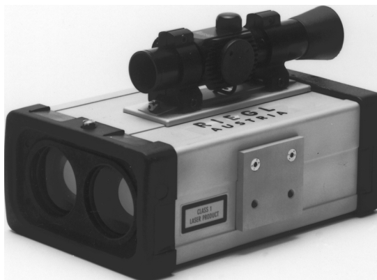
FIGURE 19.67 The Class 1 (eye-safe) LD90-3 series TOF laser rangefinder is a self-contained unit available in several versions with maximum ranges of 150–500 m under average atmospheric conditions (courtesy RIEGL USA).
