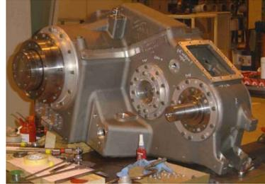
AGV prototype reducer
