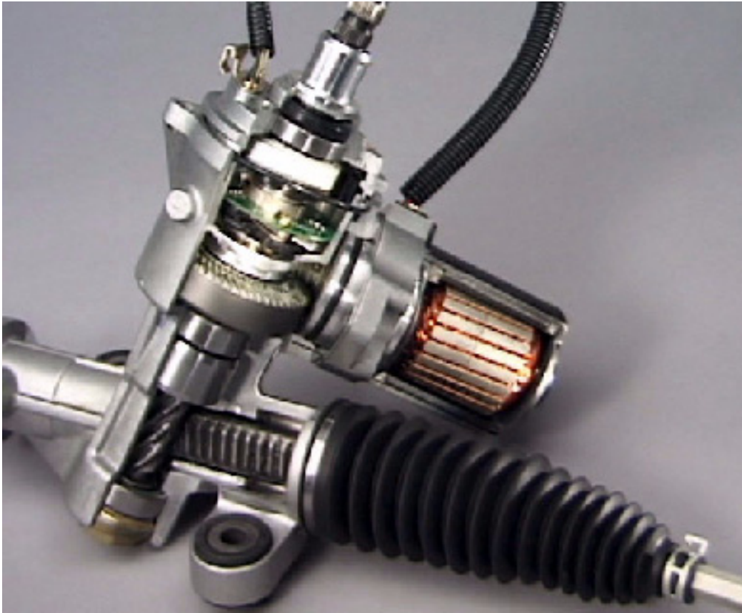
Figure 1-48 Early HEV EPS Torque Sensor, Motor, & Reduction
