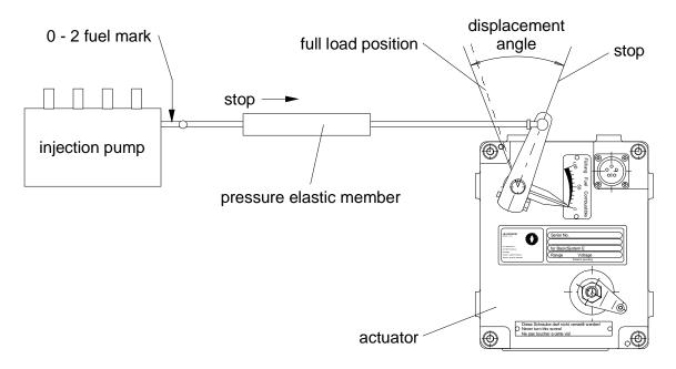
Fig. 17: Linkage for Diesel Engines
