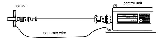
Fig. 18: Connecting a Compensation Line
