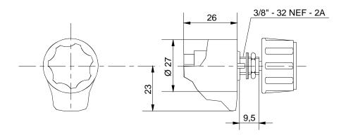
Fig. 12: Potentiometer SW 01 - 1 - b
