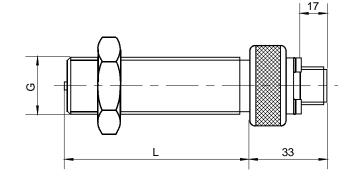
Fig. 6: Magnetic Pickup, reinforced Version
