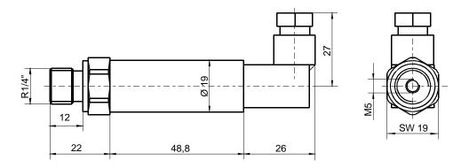
Fig. 10: Pressure Sensor with Plug Connector
