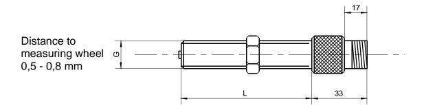
Fig. 5: Dimensions of the Magnetic Pickups
