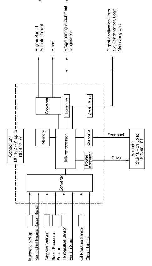
Fig. 1: General Block Diagram DG 16.2 - 01 to DG 40.2 - 01
