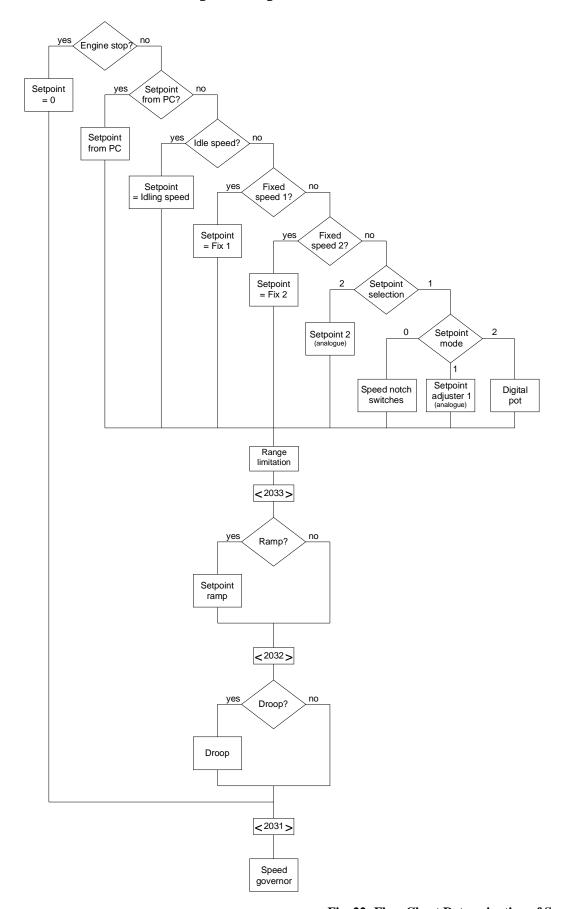
Fig. 22: Flow Chart Determination of Speed Setpoint
