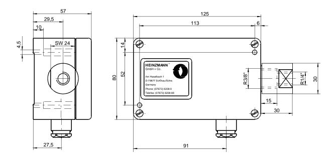
Fig. 11: Pressure Sensor with Housing
