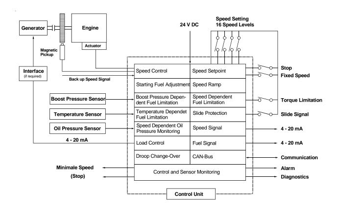
Fig. 2: Block Diagram for Diesel-Electric Drive
