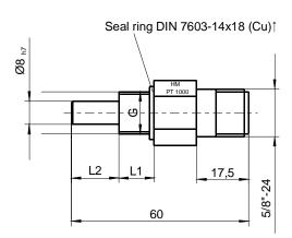
Fig. 7: Temperature Sensor TS 01 - 28 - PT 1000
