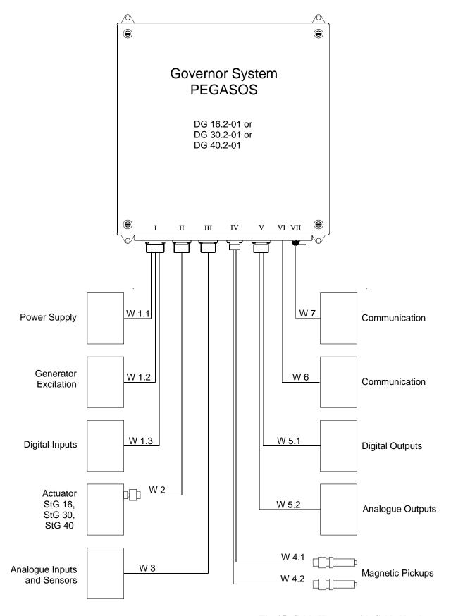
Fig. 25: Cable Harness with Cable Numbers
