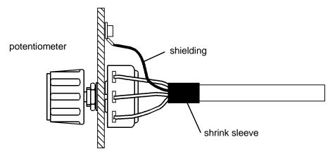
Fig. 19: Example of a Shield Installation without Plug Connectors
