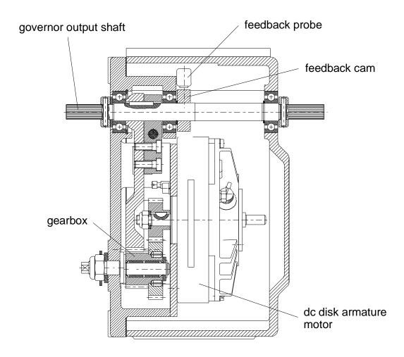
Fig. 15: Actuator Sectional Drawing
