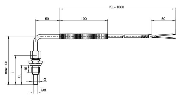
Fig. 8: PT 200 - Sensor with Cable and End Sleeves
