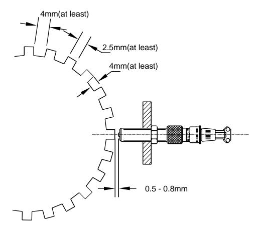
Fig. 4: Clerance of Pickup
