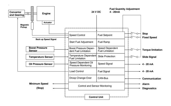
Fig. 3: Block Diagram for Diesel-Hydraulic Drive
