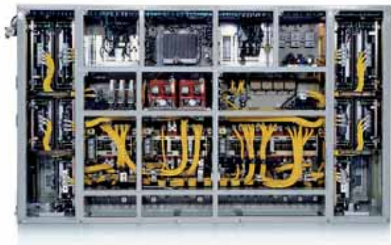
Traction converter with HV-IGBT technology
