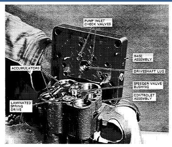
Figure 5-4. Removal of Base from Controlet
