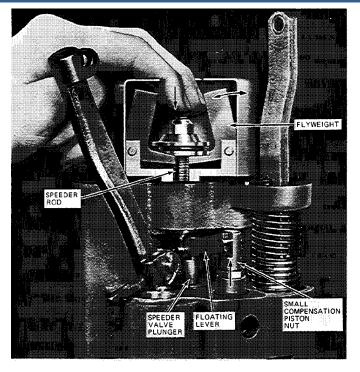
Figure 5-9. Third Check for Binding of Floating Lever
