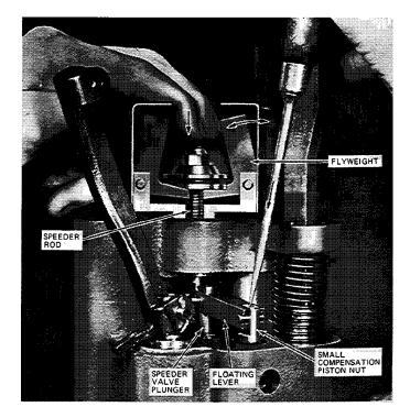
Figure 5-8. Centering Speeder Valve Plunger
