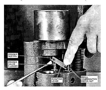
Figure 5-3. Removal of Ballhead from Controlet
