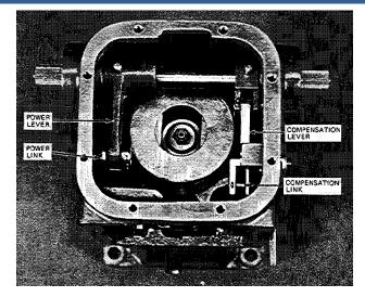
Figure 5-1. Top View of Case Assembly
