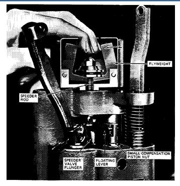
Figure 5-7. First Check for Binding of Floating Lever
