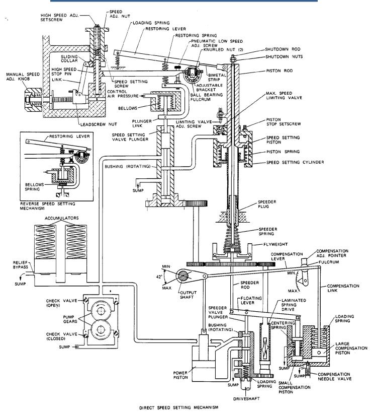
Figure 3-1. Schematic Diagram
