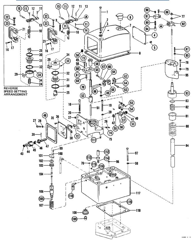
Figure 6-1. Exploded View of Column
