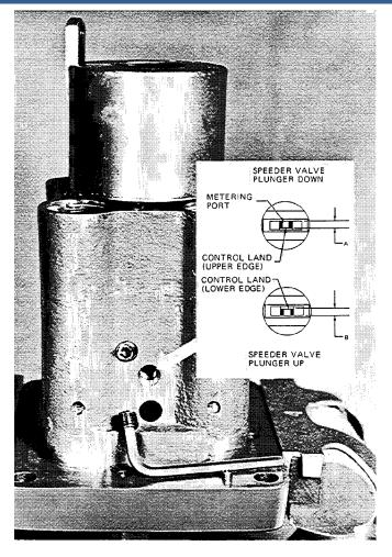
Figure 5-10. Centering Speeder Valve Plunger
