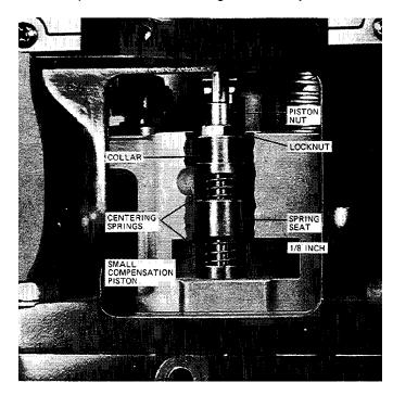
Figure 5-6. Adjusting Small Compensation Piston Centering Spring Preload
