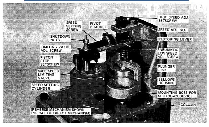
Figure 2-1. Speed Setting Adjustments
