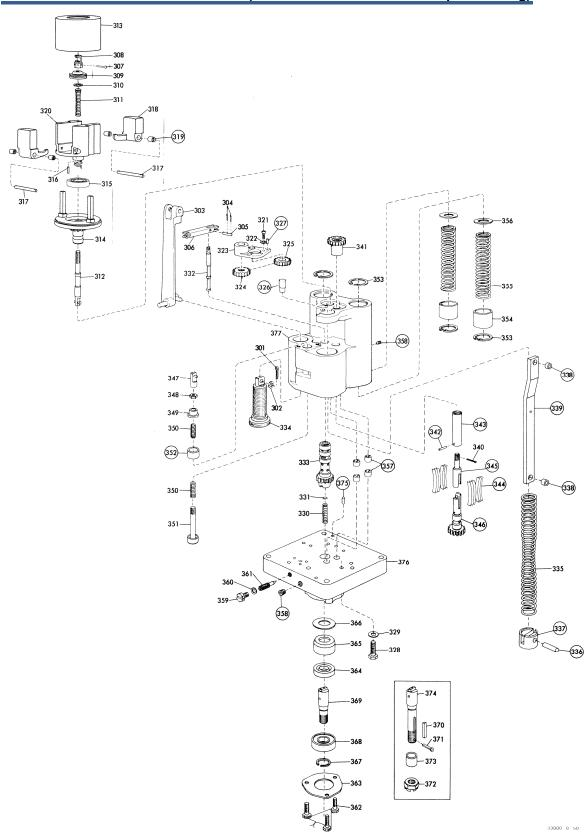
Figure 6-3. Exploded View of Controlet and Base
