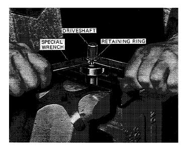
Figure 5-5. Removal of Driveshaft Retaining Ring
