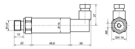
Fig. 10: Pressure Sensor with Plug Connector
