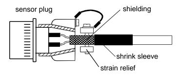
Fig. 20: Example of a Shield Installation within the Plug
