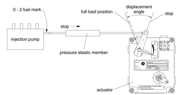
Fig. 17: Linkage for Diesel Engines
