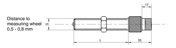
Fig. 5: Dimensions of the Magnetic Pickups
