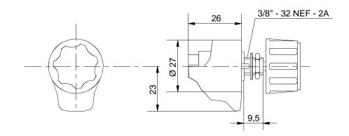
Fig. 12: Potentiometer SW 01 - 1 - b
