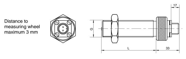
Fig. 6: Magnetic Pickup, reinforced Version
