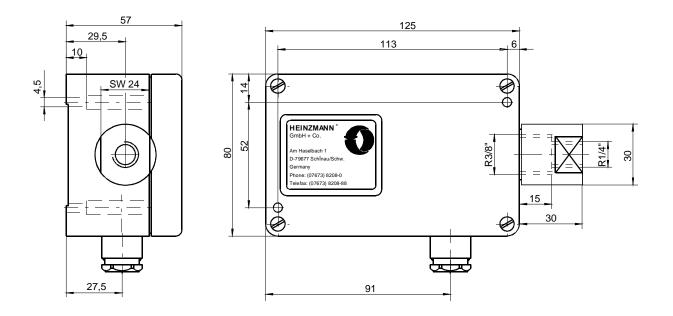
Fig. 11: Pressure Sensor with Housing
