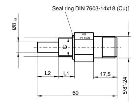
Fig. 7: Temperature Sensor TS 01 - 28 - PT 1000
