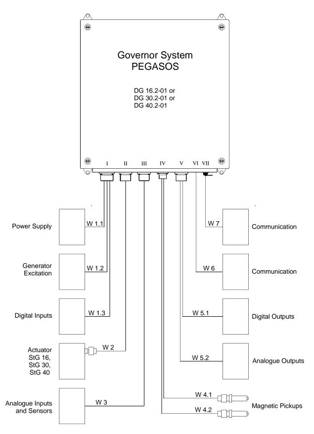
Fig. 25: Cable Harness with Cable Numbers
