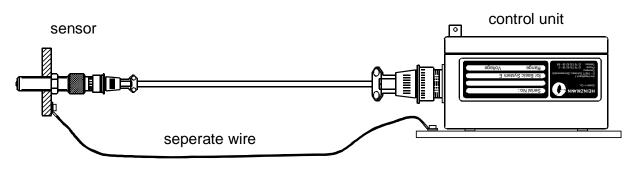
Fig. 18: Connecting a Compensation Line
