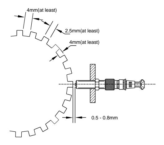
Fig. 4: Clerance of Pickup
