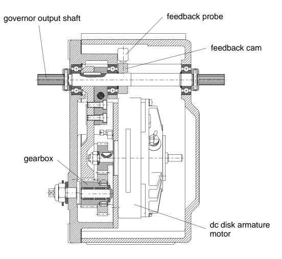
Fig. 15: Actuator Sectional Drawing
