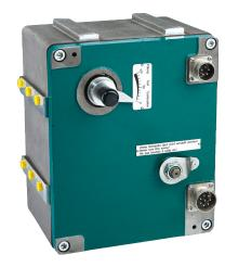
response times can be gained. In case of voltage loss a return spring ensures setting back to zero position. Optionally the actuator is available without return spring. A contactless feedback system is integrated onto the governors output shaft offering an electrical position signal to any external control unit.
