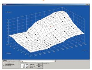
Programming characteristic maps using 3D representation, e.g. characteristic map of injection duration for magnetic valve systems, PID map, characteristic map of injection pump.
