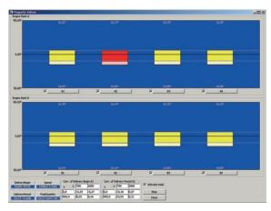
Visualisation of injection timing and injection duration for magnetic valve technology.
