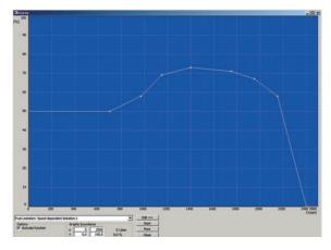
Programming curves, e.g. speed dependent fuel limitation, boost pressure dependent fuel limitation, oil pressure monitoring.
