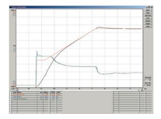
Representation of measured values vs. time. Up to ten measurements may be displayed simultaneously.
