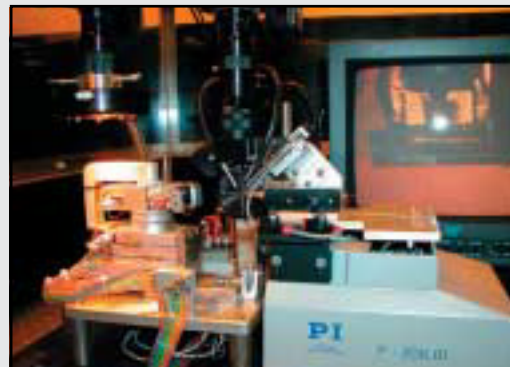
F-206 Hexapod alignment system at a workstation for automated pigtailed fiber optic devices. Printed with permission from Aries Innovations.
