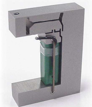
Figure 3 – DSM LPA-100 piezo-actuator uses a simple lever-arm mechanical amplification. (PZT stack is green - output is in vertical direction)
