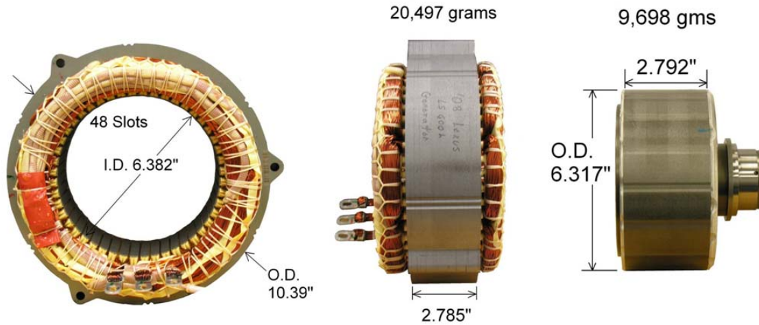
Fig. 2.71. LS 600h generator stator and rotor.
