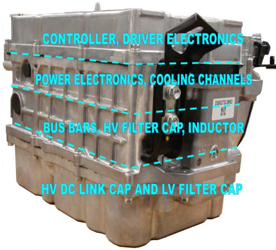
Fig. 2.3. Compartments of the LS 600h inverter and converter assembly.
