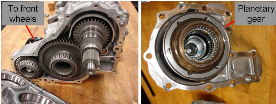
Fig. 2.63. Internal components of transfer case.
