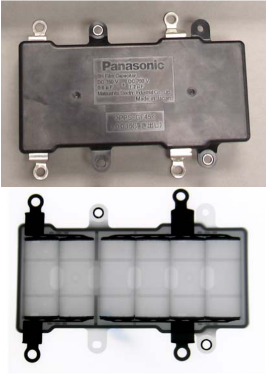
Fig. 2.14. HV filter capacitor (upper) and x-ray of module (lower).
