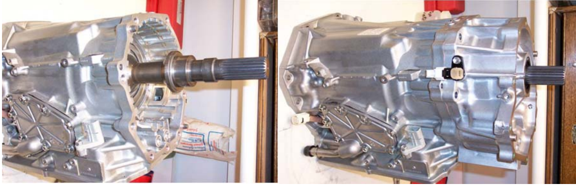
Fig. 3.2. Customized shaft installed.
