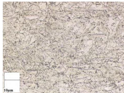
Figure 2.B-11: Micrograph of CP 800/1000 hot rolled steel.
