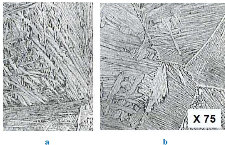
Figure 10: a: Near \alpha -Ti alloy quenched from \beta -phase field, b: Near \alpha -Ti alloy air-cooled from \beta -phase field
