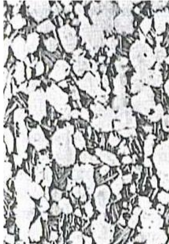
Figure 9: Air-cooled from \alpha+\beta phase field, having white primary \alpha -phase and Widmanstätten \alpha - \beta structure
